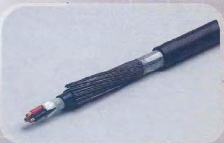
Steel Wire Armored Cable after 2 week exposed in the air. Rust occurred at the armor.
