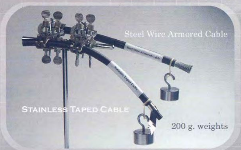
STAINLESS TAPED CABLE after 2 week exposed in the air. No rust occurred.
