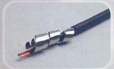
STAINLESS TAPED CABLE after 2 week exposed in the air. No rust occurred.
